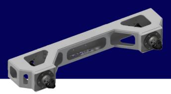
Most Beluga VBS' can be delivered with ROV docking. The ROV docking enhance the ROV ability to control the VBS without strain on the manipulators. The ISO Standard docking probes is a field proven and failsafe design. C/C 1050 mm
