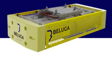
The versatile Variable Buoyancy - ROV Skid allows a wide range of WROV to increase payload and adjust their own buoyancy by operating a VBS pump and adjust water level inside the integrated VBS tanks. This enable the ROV operators to preform lifting operations with the ROV up to 1000Kg without support from crane or any other lifting solution.
